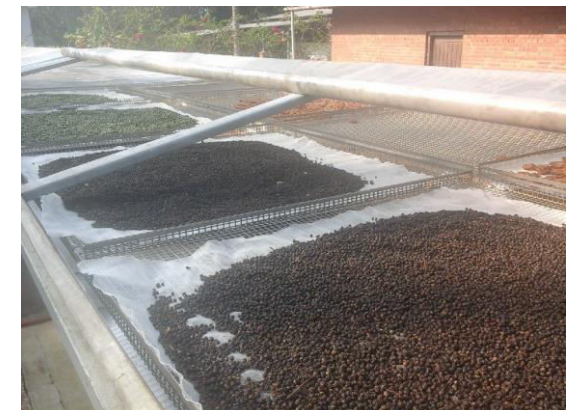
Solar drying of spices- nutmeg and mace
